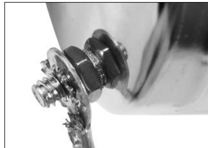
Step 15 - Slide Ring Terminal Wire Assembly onto Stud & Lock Washer over Ring
