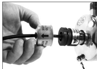
Step 2 - Remove End-Cap
