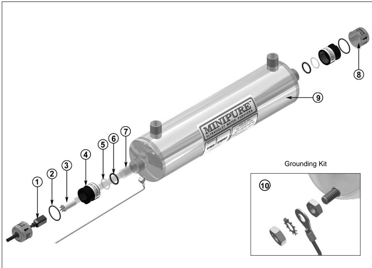
Table 5 - Replacement Parts MIN-6 120v 50/60Hz using ballast no. 10-0508A
