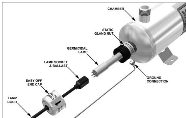
9. Unpack the lamp and ballast. While holding lamp end, carefully push lamp socket on. Carefully slide lamp straight into the quartz sleeve, without angling. Push the end cap on, over the static gland nut.
